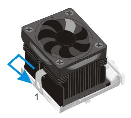
3. Clip-on the second lock and please make sure not to damage/scratch the board.
